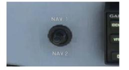
NAV 1 frequency is set from the GPS and NAV 2 frequency from the secondary radio unit.
