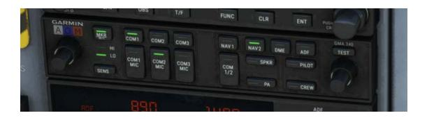
It features two double knobs to set pilot/copilot intercom volume and squelch level, and the following buttons:
