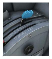
In case of regulation failure, pressure drop results in automatic transition to high pitch.
