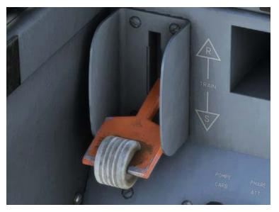
Then, you need to pull emergency gear lever to let the landing gear going down.
